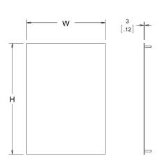
Front plates are 14 gauge aluminum with clear anodized brushed finish. Mounting hardware included.
